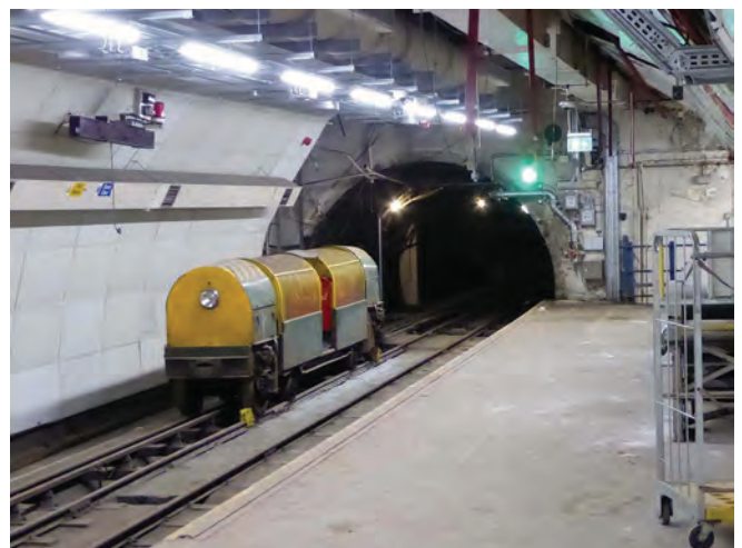
An old maintenance train, constructed to carry engineers, stabled at the platform
